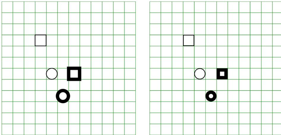
Fig. 5.23. Left, standard mode, elements grow into both directions (setting Outerlimits=0). Right, elements grow only to the inside (setting Outerlimits=1).
